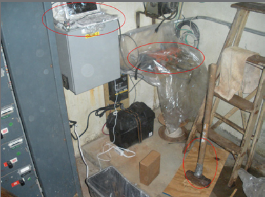
Fig. 7. The arrangement of the two sensors. Both the example client and the MIKB sensor are visible. Also seen here is the sledgehammer used to simulate seismic activity for testing purposes.
