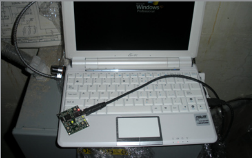
Fig. 5. An example client. The accelerometer device is seen here connected to the USB port on an example laptop.
