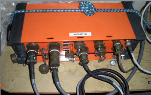
Fig. 6. Sensor MIKB. This is one of the sensors in the Southern California Seismic Network, and is designated MIKB since its location is in the basement of Millikan Library on the Caltech campus.
