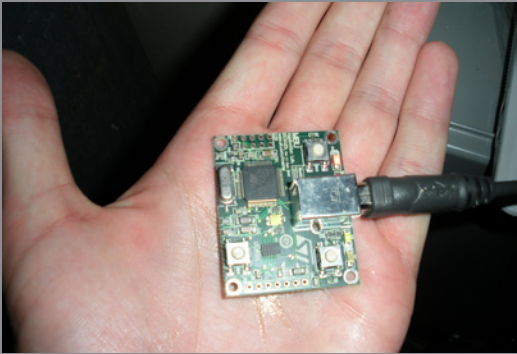
Fig. 4. The accelerometer device, before it has been connected to a computer.
