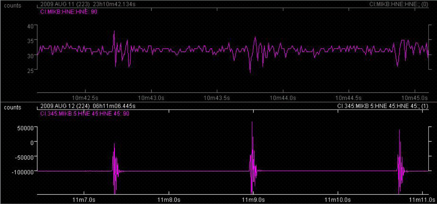
Fig. 8. The impact of the sledgehammer, as detected by the two sensors. The signal detected by our sensor is much less clean.
